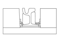
The components of the chamber completely wrap the rail in its lower part and its sides, thus meeting the insulation needs required by the rails in urban routes:
